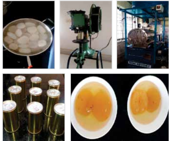
Fig.1 Process of canning: a) preparation of PTFE, b) filling and double seaming, c) heat processing of cans, d) after canning and e) finished product at 180th day
